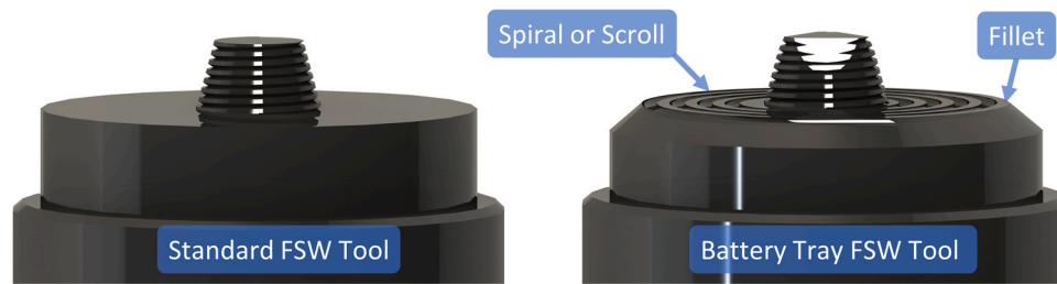
Fig. 16. Battery tray FSW tool compared to the typical FSW tool.
